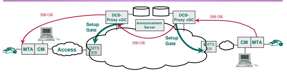
◆ 200 OK conveys call parameters and (gate id) to originating MTA
